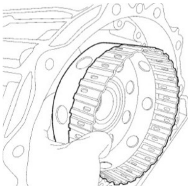
Fig. 10 K2 Clutch Hub
