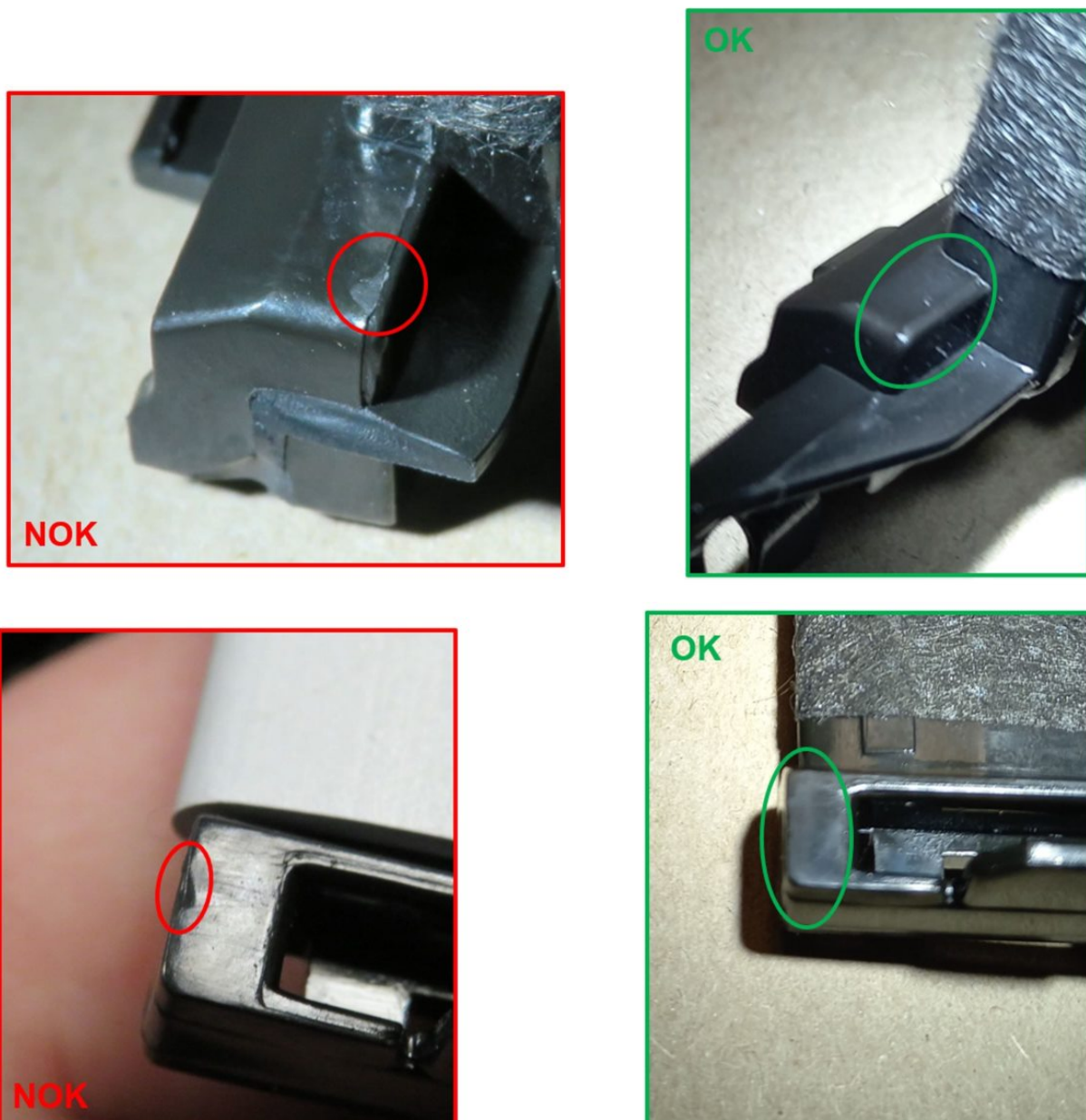
Figure 3 Damage of the sunroof blind slide shoes due to contamination check
