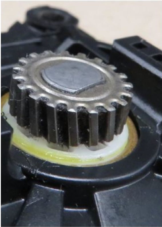
Figure 8 Electric drive motor pinion inspection
