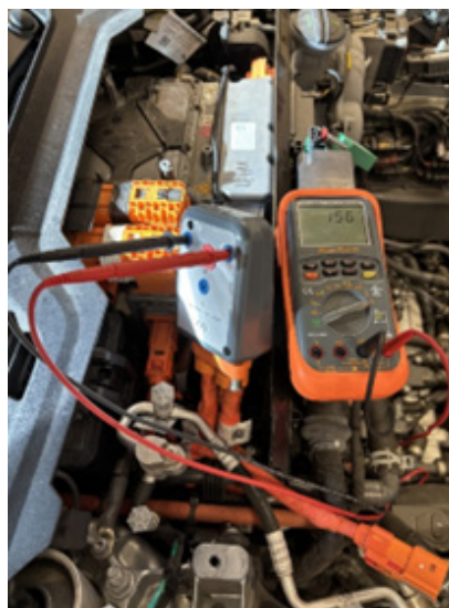
Figure 3 - Measuring Capacitance on Front PE
