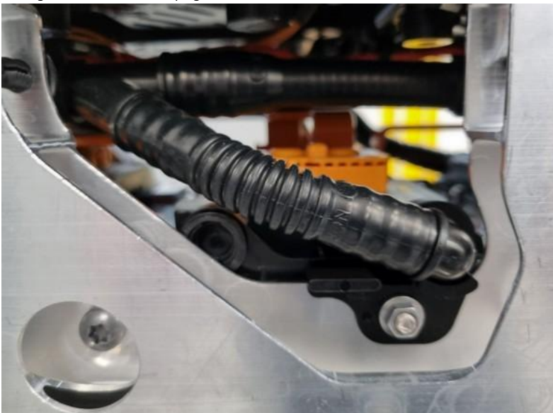
Cooling manifold and module plug
