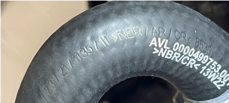
Pump inlet hose marking
