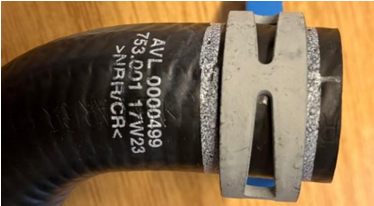
Pump inlet hose marking
