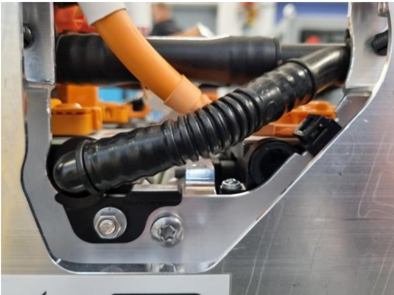
Cooling manifold and module plug
