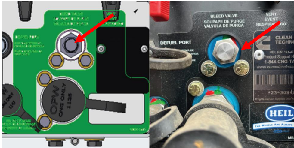
Figure 5. Bleed Valve on FMM
