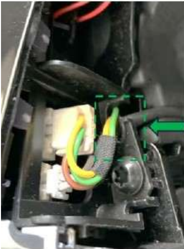
Figure 2. Correct wire routing on left side.
