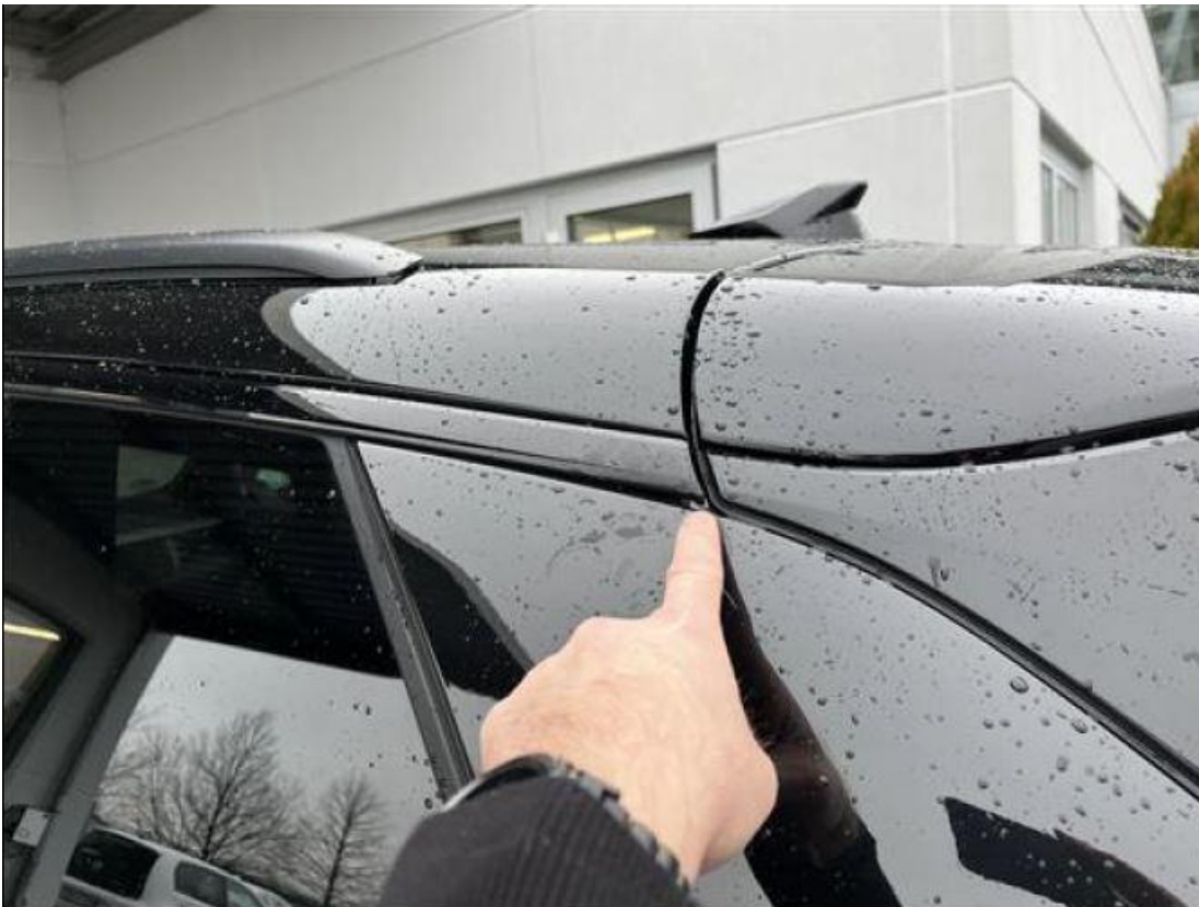
Figure 1. Example of the protruding trim.
