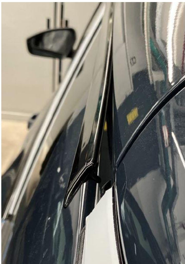
Figure 2. Example of the protruding trim.
