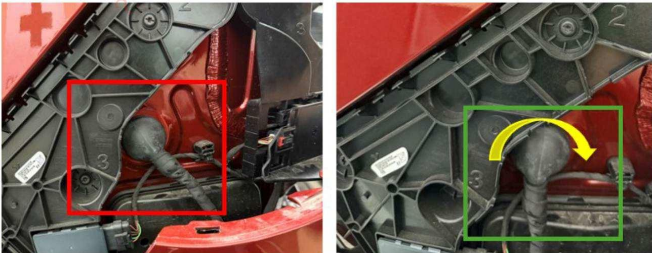
Figure 5. Left – factory grommet orientation. Right - bumper wiring harness grommet in 6 o'clock position.
