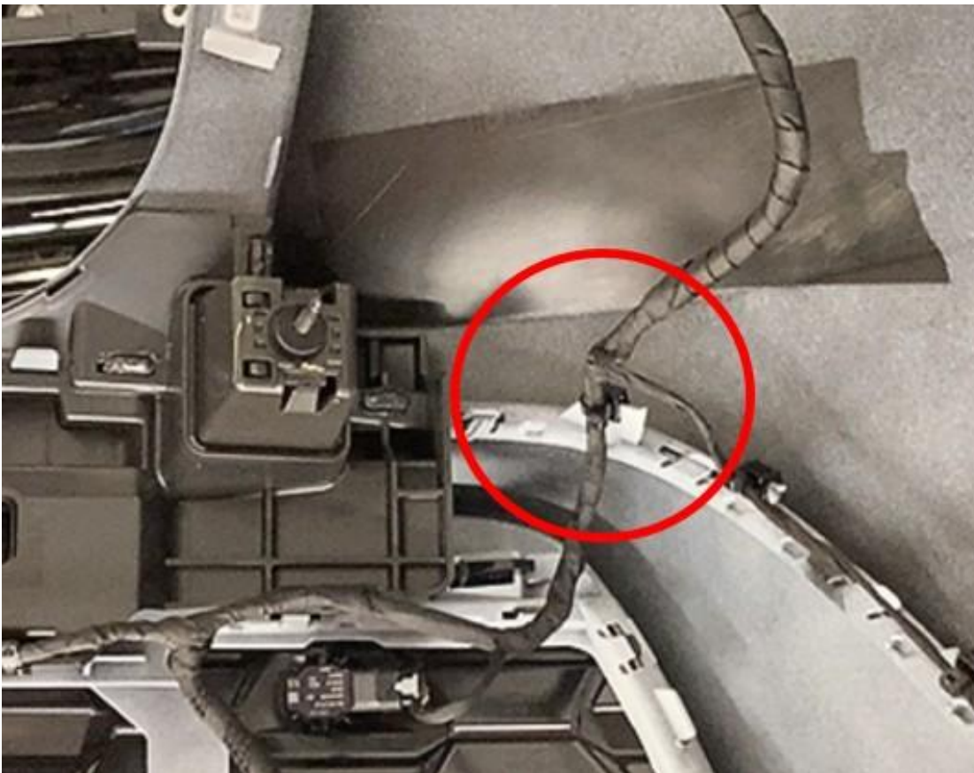
Figure 3. Position of cable tie with clamping base
