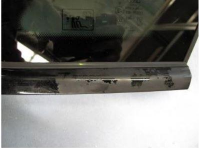
Figure 2. Coat peeled off.
