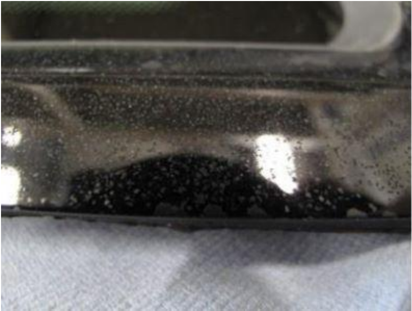
Figure 3. Spots of additional coating.
