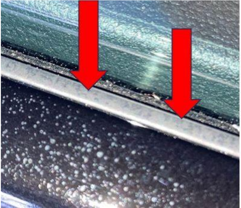
Figure 5. Marks forming caused by applied liquid.
