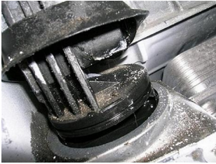
Figure 2. Dust cover lifted to view the sealing area.
