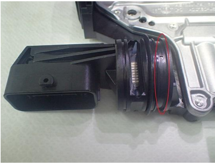
Figure 5. A seal fitted as standard Modified state after performing TSB (Figure 6).
