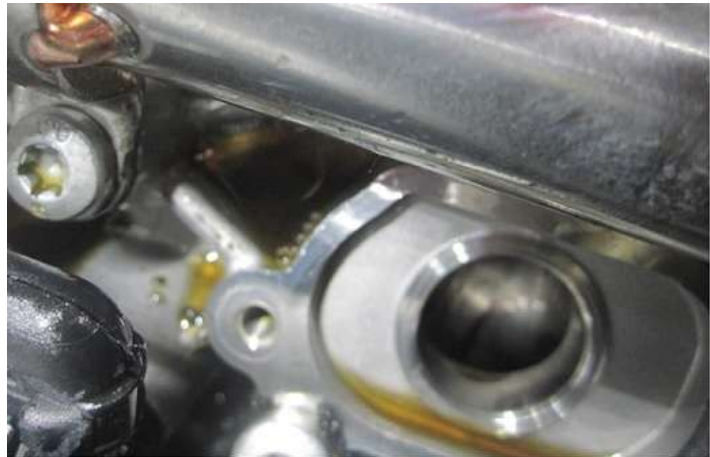
Figure 2. Oil in the Audi valve lift system.
