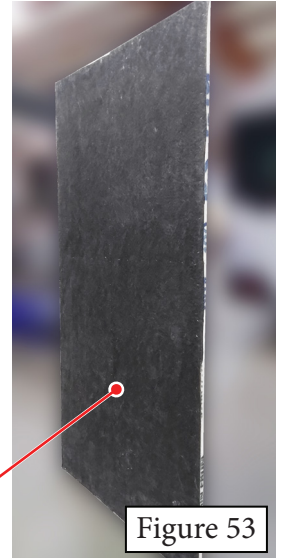
FELT COVERED PLYWOOD
