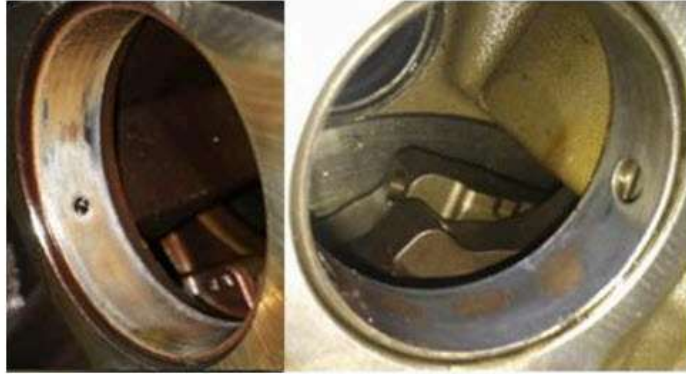
Delamination (Exposed copper)
