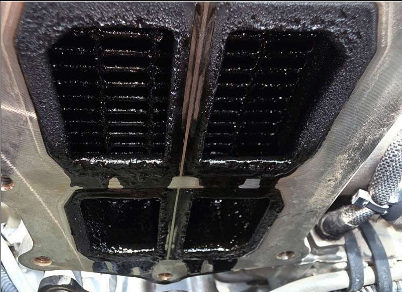
Example of soot/fuel mixture in the EGR system. Note, this example shows the EGR cooler.
