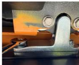
Tighten accessible bolt to Locate Striker on door while closed
