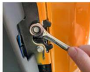
Loosen Latch Bolts
