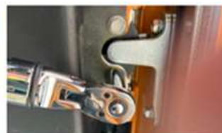
Torque to 6-8Nm w/ Door Fully Latched
