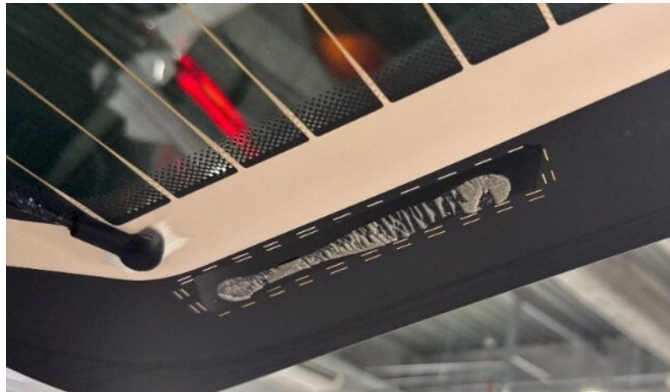
Fig. 5 Liftgate Damper Location - Missing Damper
