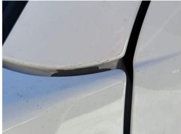
Examples of paint peeling on the left A-pillar
