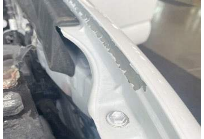
Examples of paint peeling on the front inner fender edge (can be seen with the hood open)
