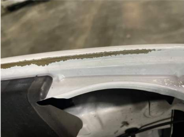
Examples of paint peeling on the front inner fender edge (can be seen with the hood open)
