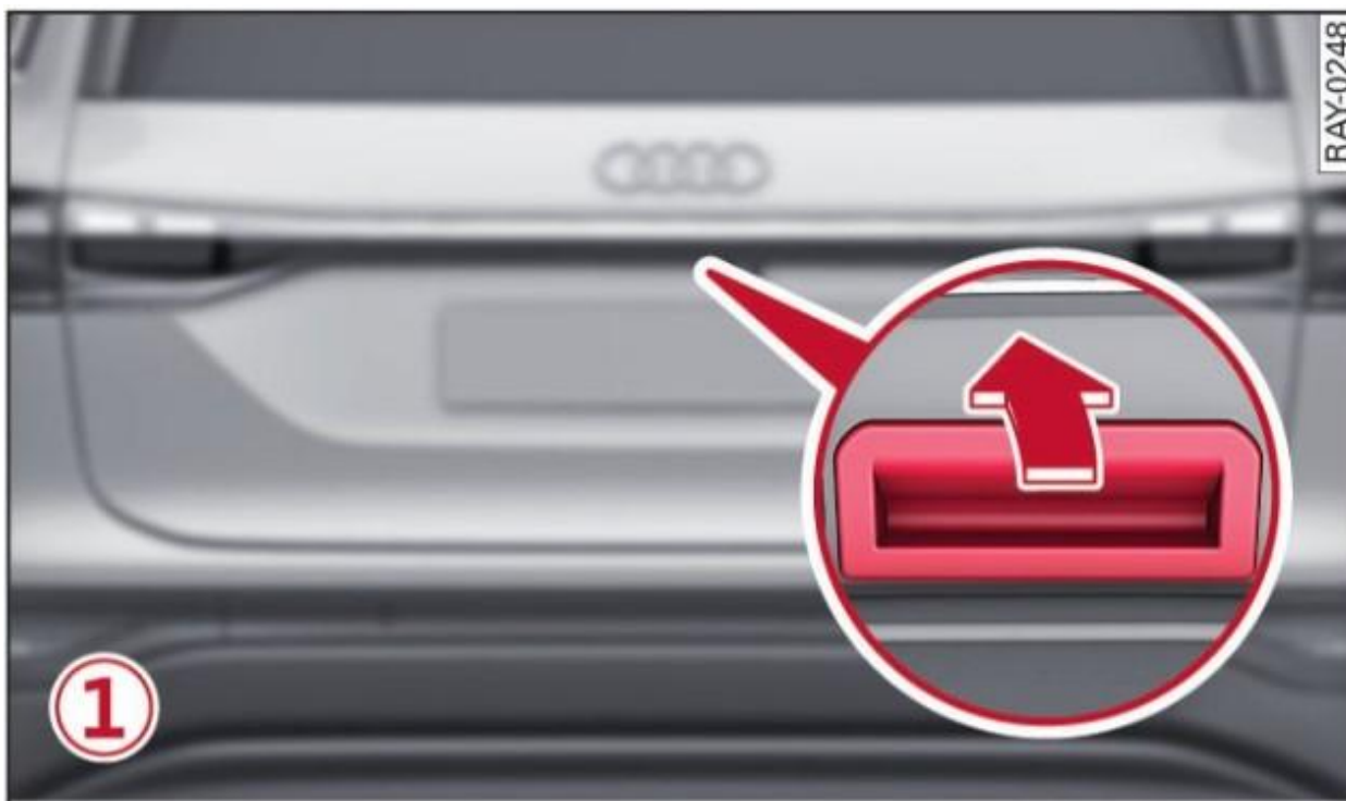
Figure 2. Electric rear lid lock actuation button.
