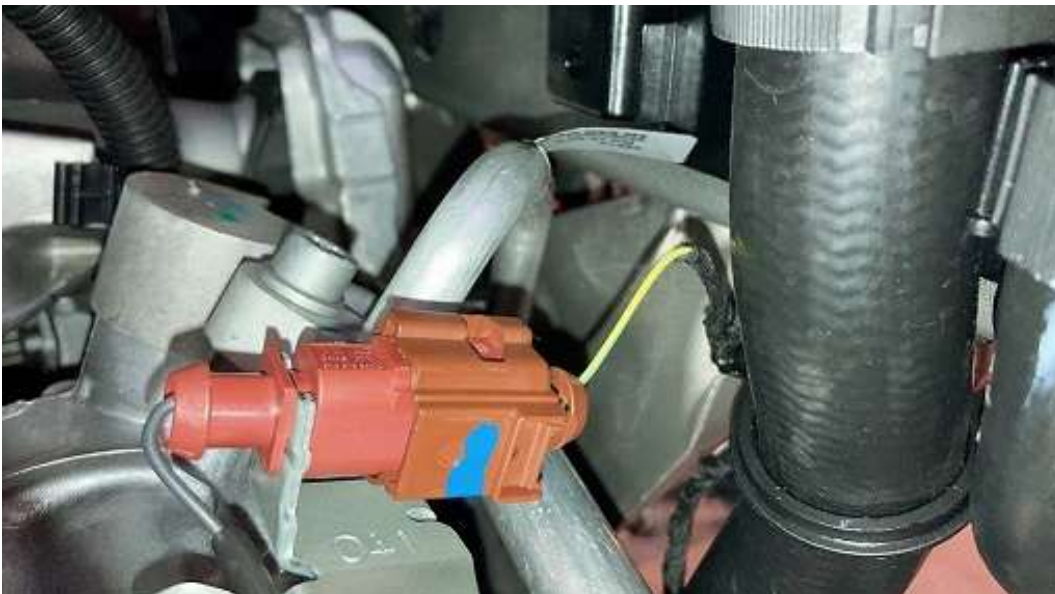
Figure 2. Connector in its repaired state.
