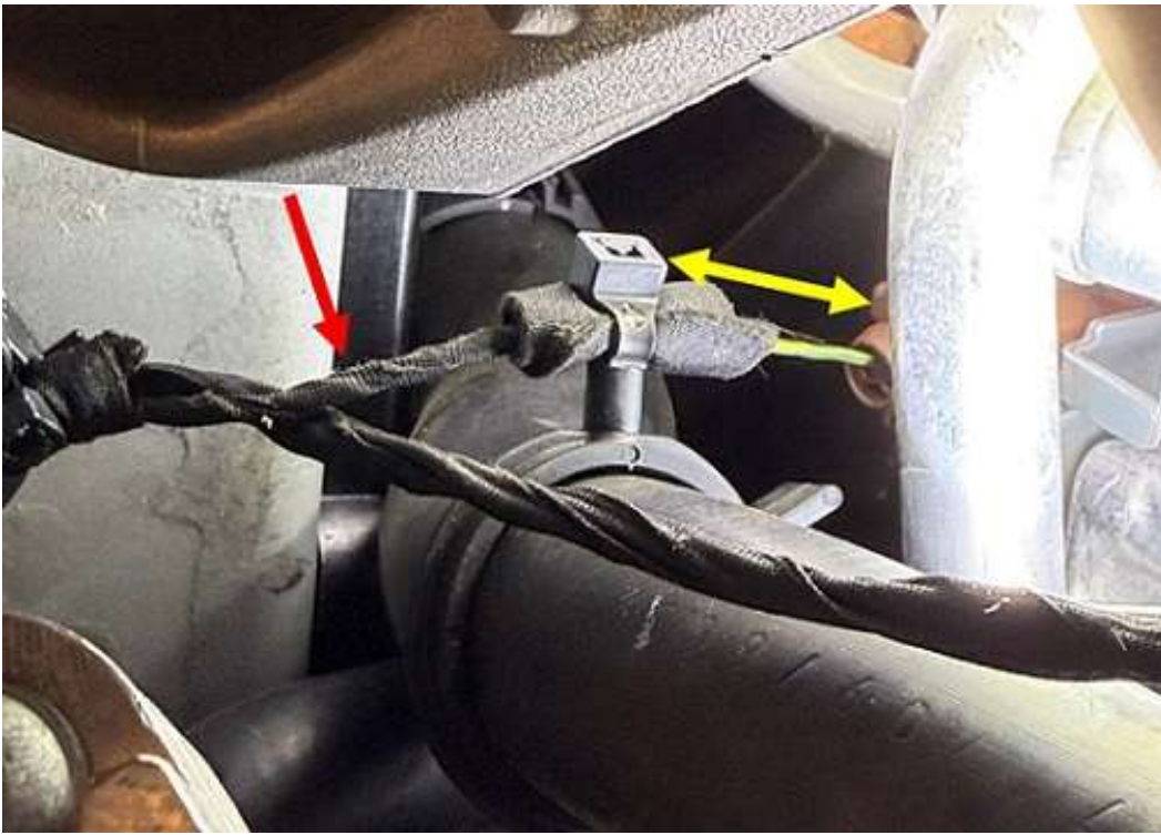
Figure 1. The position for the crimp connector is marked with the red arrow.
