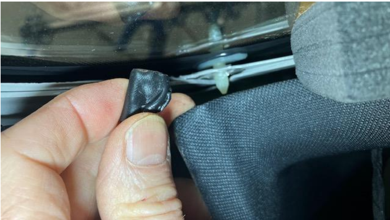
Figure 2. Use butyl adhesive sealing cord as pictured.
