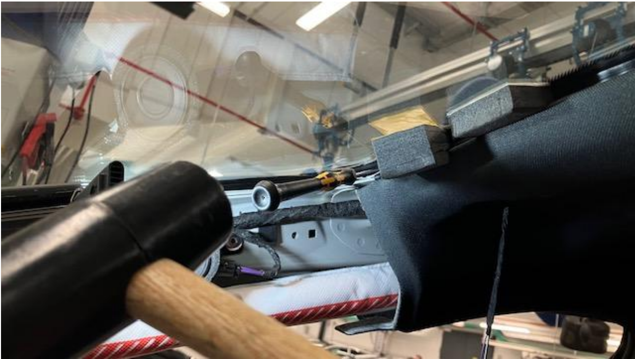
Figure 6. Carefully knock out the windscreen pin with a sharp screwdriver.
