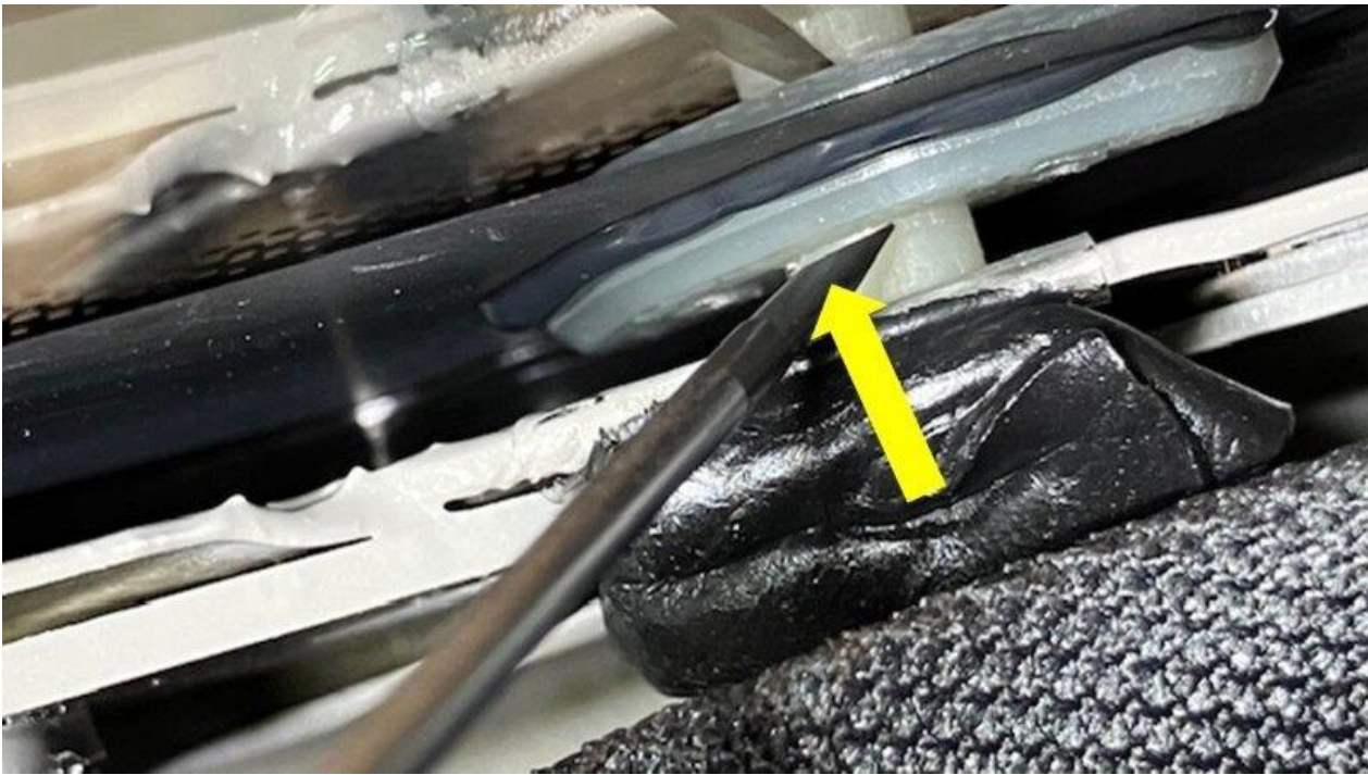
Figure 5. Carefully knock out the windscreen pin with a sharp screwdriver.
