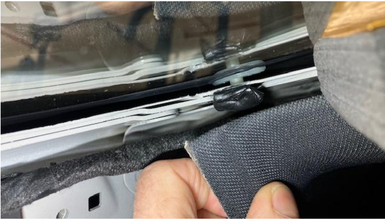
Figure 3. The butyl adhesive sealing cord covers the pin.
