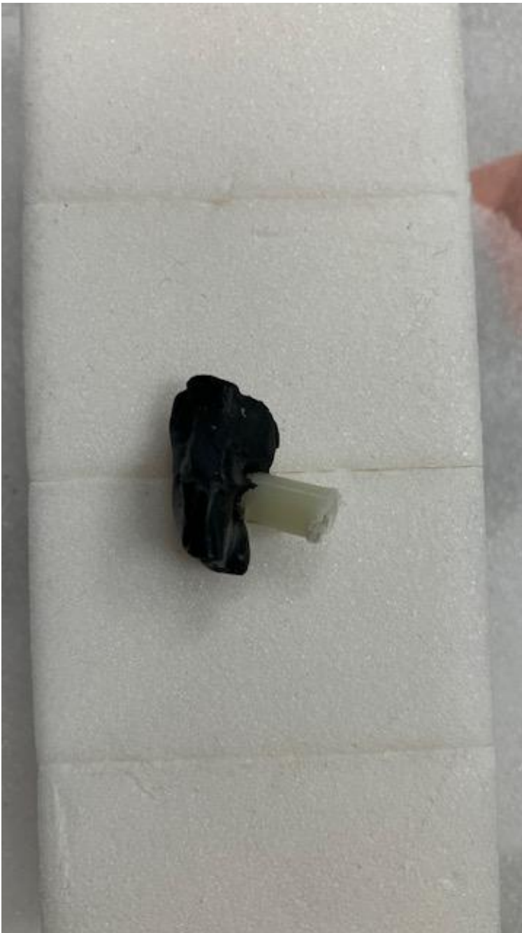
Figure 7. Windscreen pin with butyl adhesive sealing cord after being removed.
