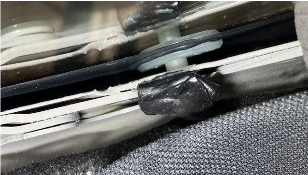
Figure 4. The butyl adhesive sealing cord covers the pin.
