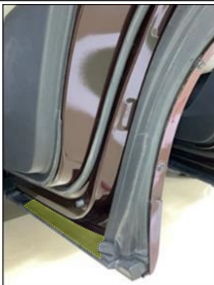
Attachment Location (on rear door lower garnish)
