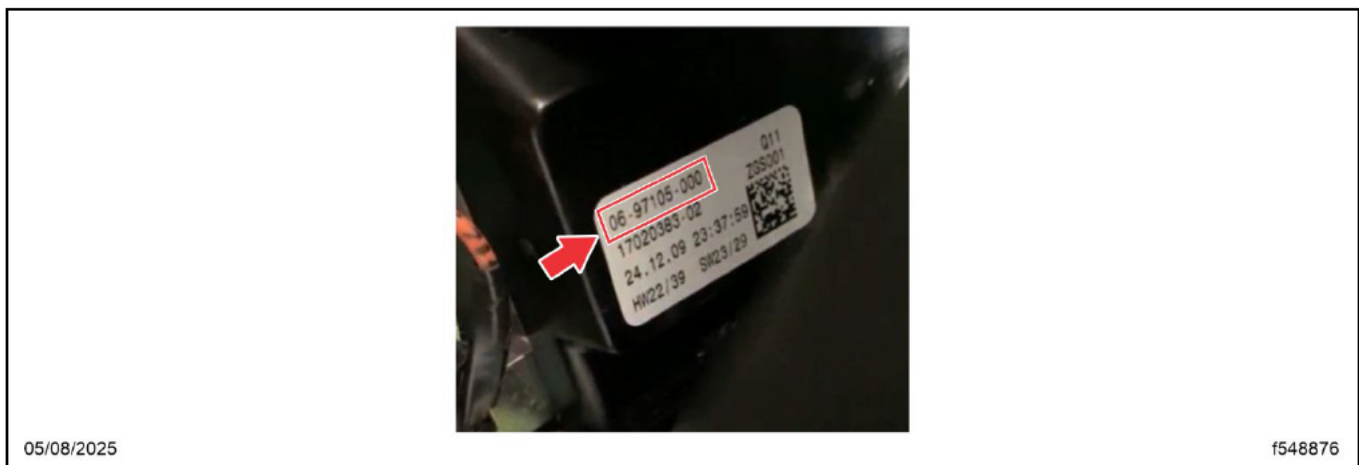
Fig. 1, Stalk Switch Part Number on the Manufacturer's Label
