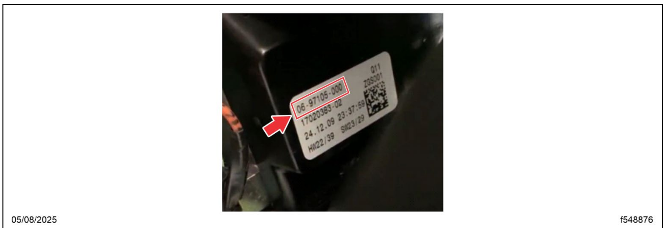
Fig. 1, Stalk Switch Part Number on Manufacturer's Label
