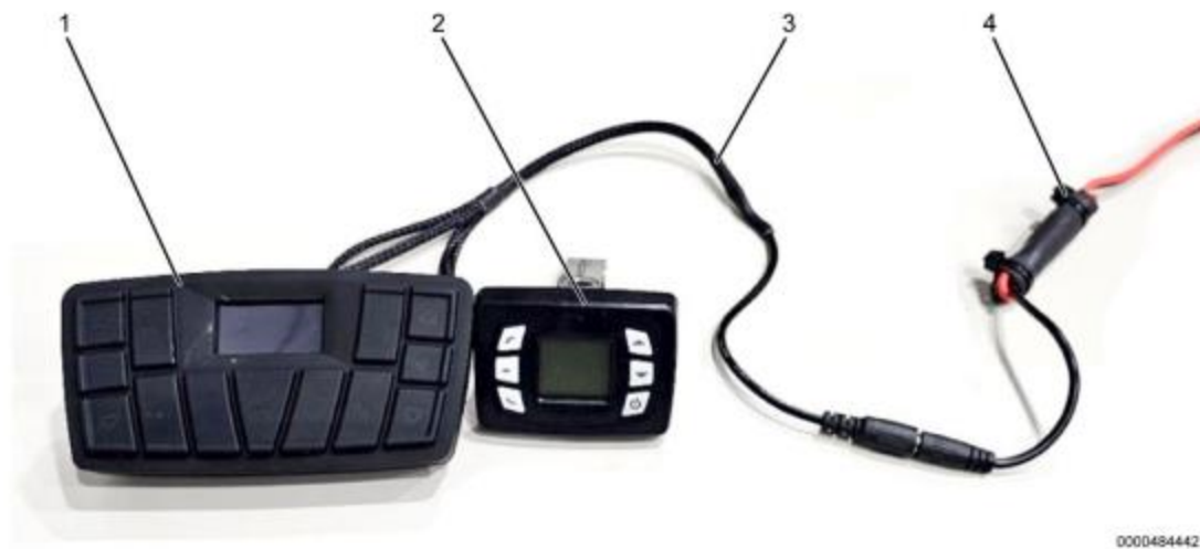
Figure 1. A/C Control Module Harness (Front View)
