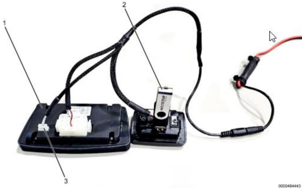
Figure 2. A/C Control Module Harness (Rear View)
