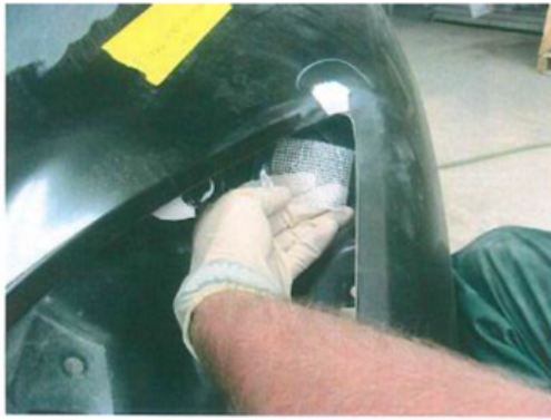
Cut mesh to cover inside surface around crack
