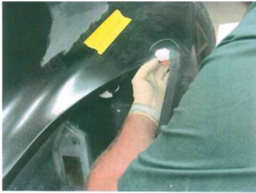
Put tape upside down and layer Fibril and mesh on sticky side of tape so it will stick to under side of hood
