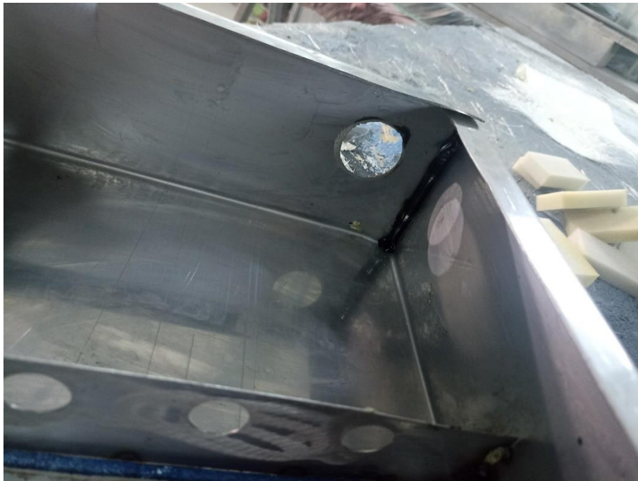
Figure 2 – Application of Sealing Compound
