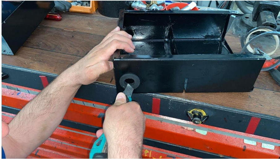
Figure 4- Application of Grommet
