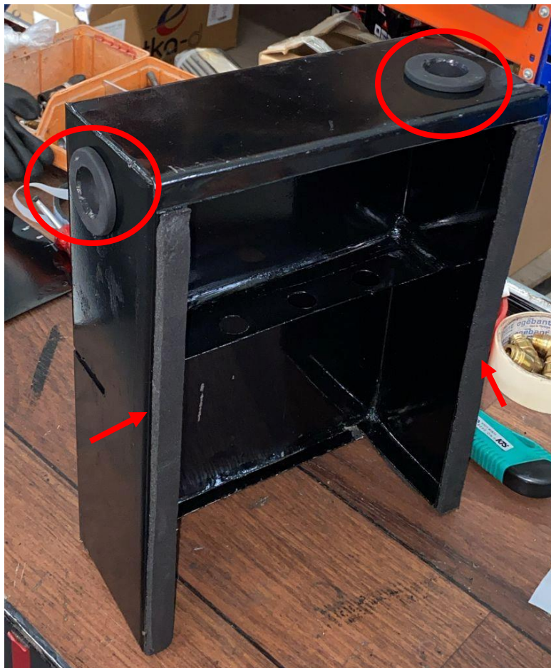
Figure 5- Application of Grommet to Cable and Hose Holes
