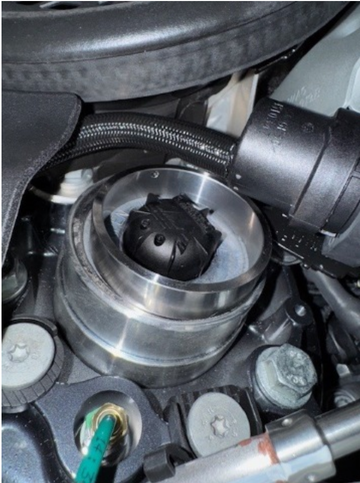
Figure 5. NOK check tool fitment
