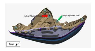
Photo is showing two adjusting knobs, but **ONLY** the height adjustment knob (green arrow) needs to be adjusted.
