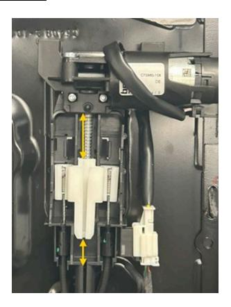
This design improvement ensures the seat back latches and headrest will release even when the actuator is experiencing a low voltage condition.
