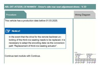
To install the new 52 20 5 B6C 6A1 into a vehicle built <u>prior</u> to March 28, 2025, you must replace the headrest actuators in both the drivers and passengers third-row seats at the same time AND perform ISTA/P conversion "Replace 3rd row actuator". This will add +AA3S into the Vehicle Order to reverse the spindle drive direction.
