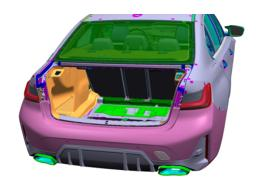
3. Remove the left and/or right-side trunk wheel arch trim panel (highlighted in orange) following the repair instructions listed in ISTA/AIR 51 47 151.
