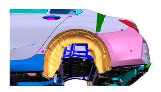
1. Remove the left and/or right wheel and wheel arch trim panel (highlighted in orange) following repair instructions listed in ISTA/AIR 51 71 041.
