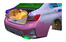
4. Remove the insulating pad (highlighted in orange in the photo).
