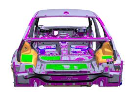
While driving on a smooth and/or uneven road, a "cracking" sound is heard from the rear wheel arch area (highlighted in orange) on either the right or left side.
