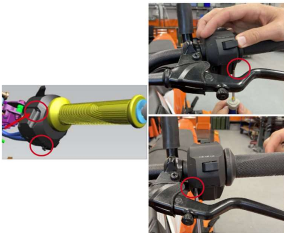
Fig. 4 – Remove LH switch control from handlebar
