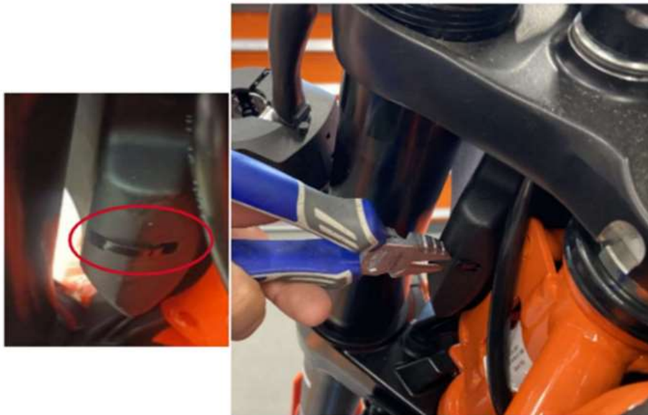
Fig. 3 – Remove cable tie on dashboard support
