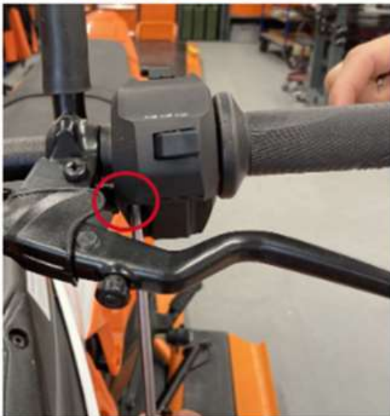
Fig. 6 – Assembling of new LH switch control
