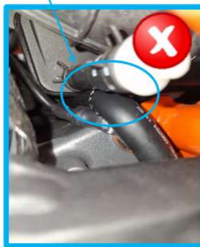
Fig. 3 – engine breathing pipe NOK
