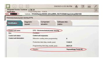
1. Verify a TKPS EPS is installed via ISTA control unit functions (G20, G22, G23, G26 and G42 only).
