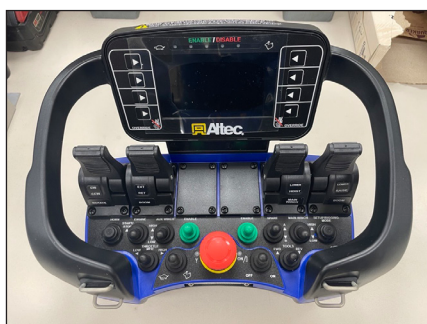
Auxiliary Winch and Articulating Jib Joysticks Not Installed
