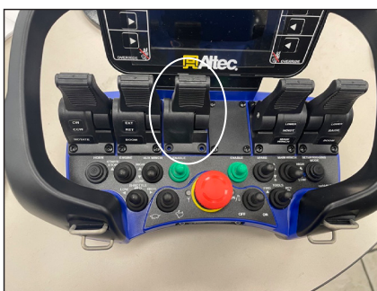
Auxiliary Winch Joystick Installed
