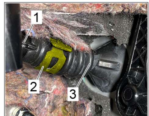
Correct installation of hose clamp
