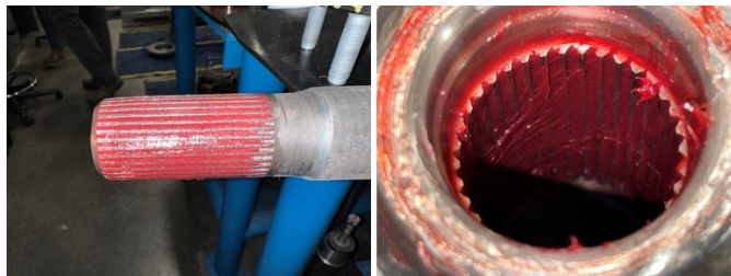
Fig. 3 Lubricated Axle Shaft/Hub splines
