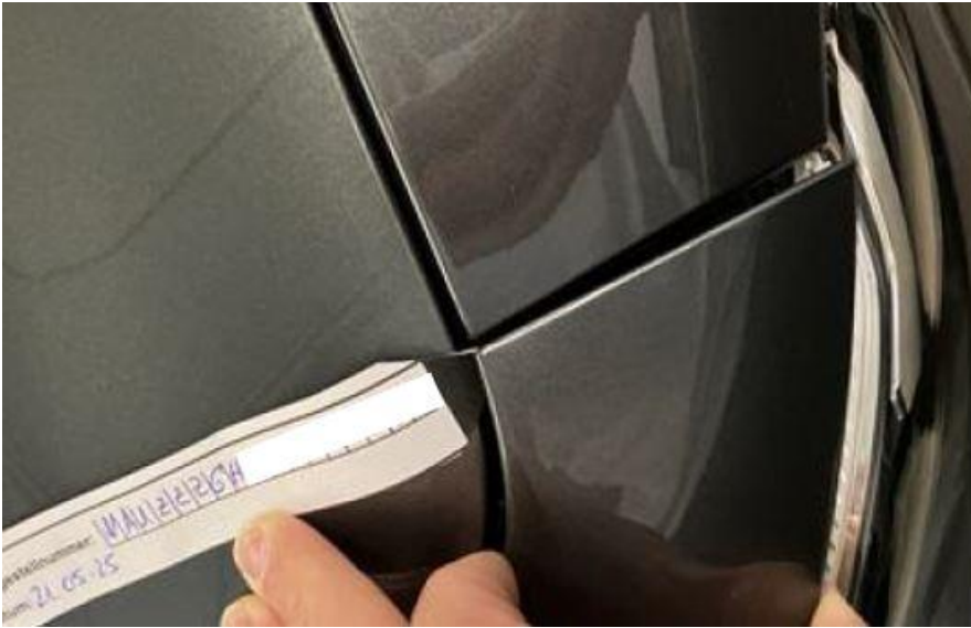
Figure 1. Example of the bumper cover protruding past the wing.
