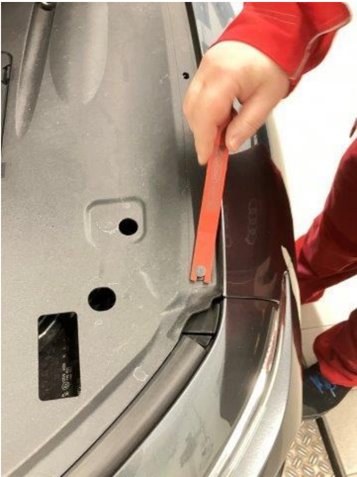
Figure 2. Loosening the inner trim.
