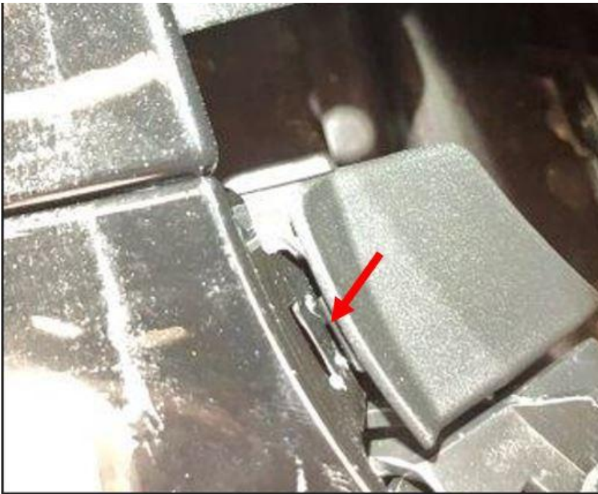
Figure 5. Image shows the area where the securing strip is clipped to the bumper cover.
