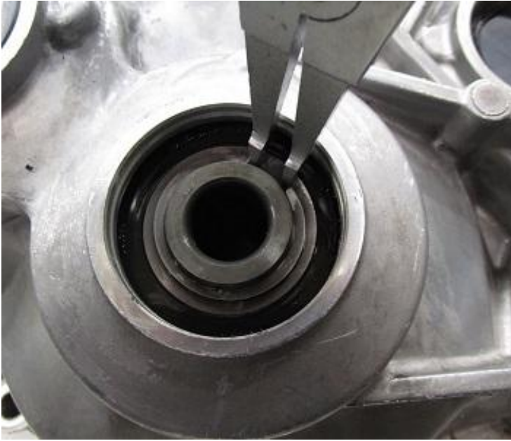
Figure 3. Removing the retaining ring for the inner ring of the intermediate shaft (example).
