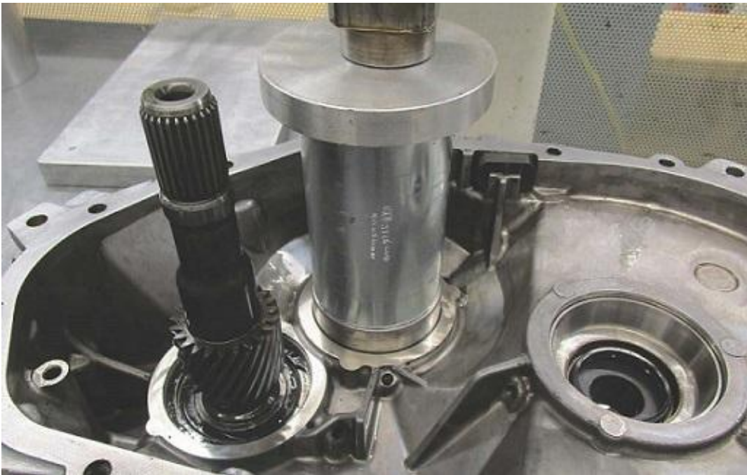
Figure 14. Pressing in the new bearing for the intermediate shaft with tube -3146-.
