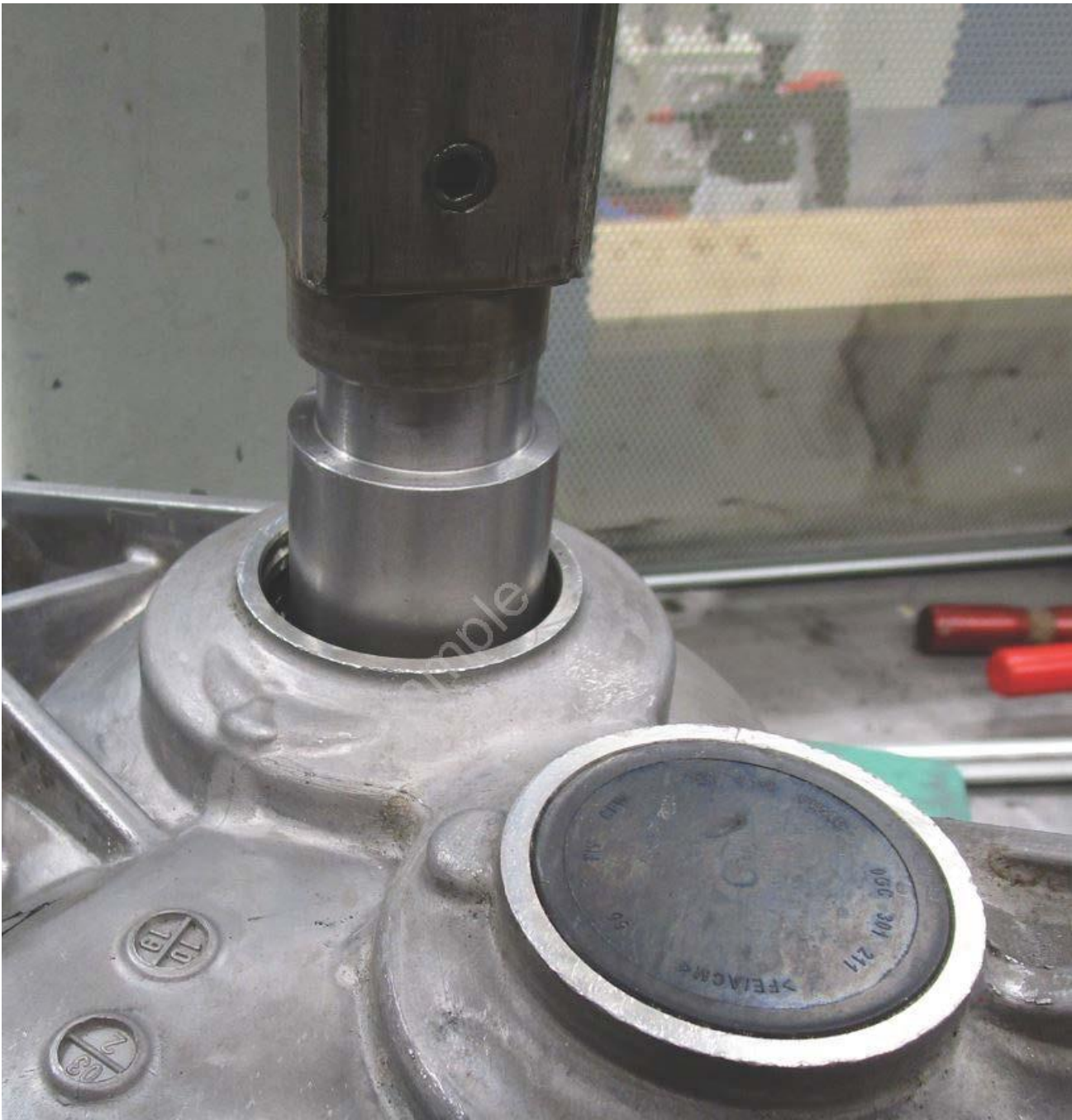
Figure 10. Pressing out the bearing for the intermediate shaft (example).
