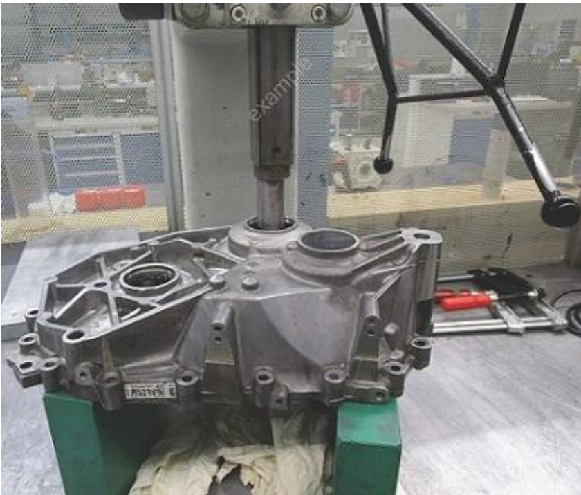
Figure 8. Pressing out the intermediate shaft (example).
