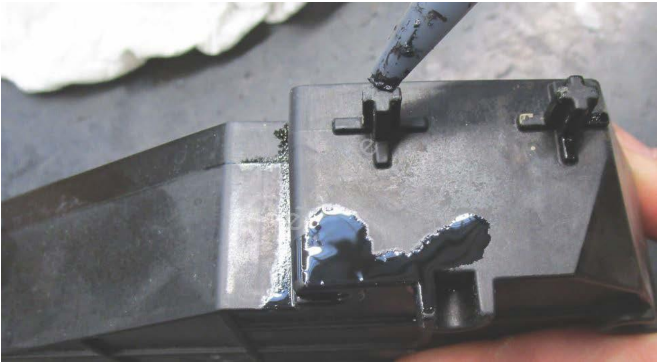
Figure 20. Lightly applying silicone sealant to the attachment point (example).
