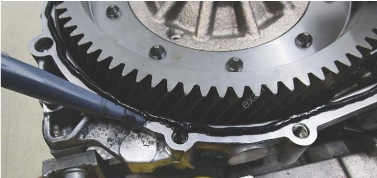
Figure 17. Applying silicone sealant all around the sealing surface of the intermediate housing (example).
