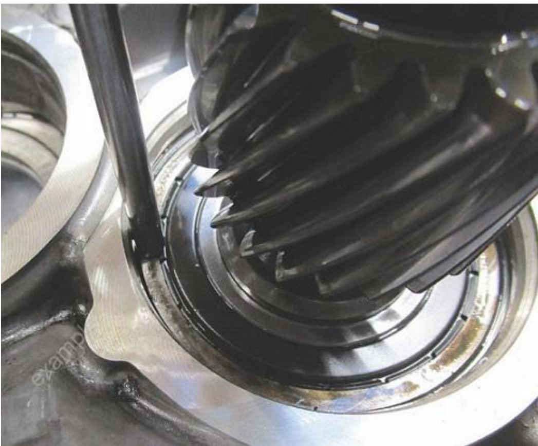
Figure 12. Driving the bearing for the drive shaft in deeper (example).
