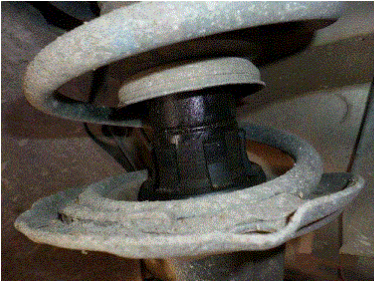
Figure 3) Not a leaking shock/strut
