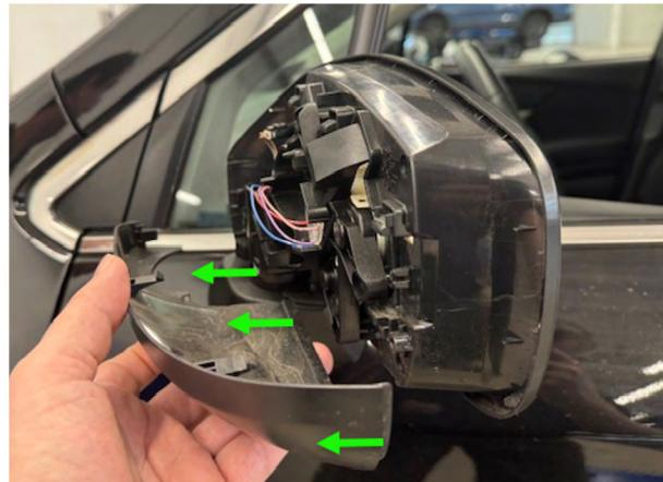
**STEP 4:** Remove the mirror turn signal lens.
