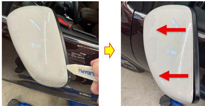
**STEP 3:** Remove the lower cover cap by pulling straight back
