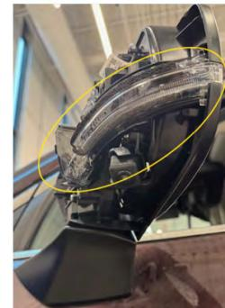
**STEP 8:** Remove the 3 screws securing the mirror surface actuation unit to the mirror housing and release the wires from retaining hook.
