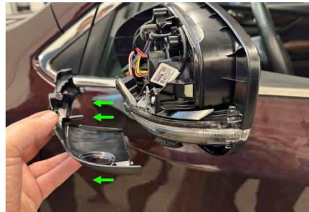
**STEP 7:** Remove the mirror turn signal lens.
