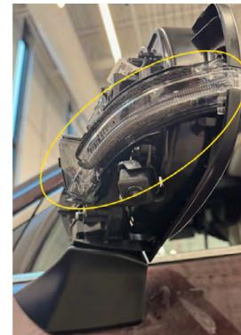
**STEP 5:** Remove the 3 screws securing the mirror surface actuation unit to the mirror housing and release the wires from retaining hook.
