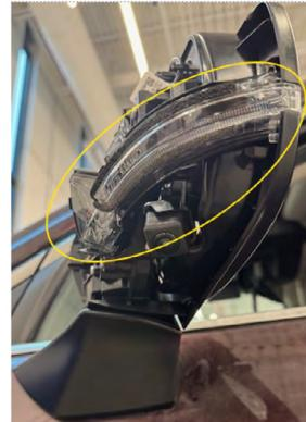
**STEP 5:** Remove the 3 screws securing the mirror surface actuation unit to the mirror housing and release the wires from retaining hook.
