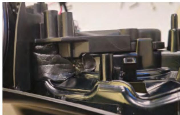
**STEP 10:** Once the areas are packed with sealer, reinstall the glass and ensure there are no obstructions. Confirm the mirror has a full range of motion. Once this is confirmed, reinstall the turn signal lens. Ensure the camera grommet correctly is in place, then install the lower cap cover followed by the upper cap cover.
