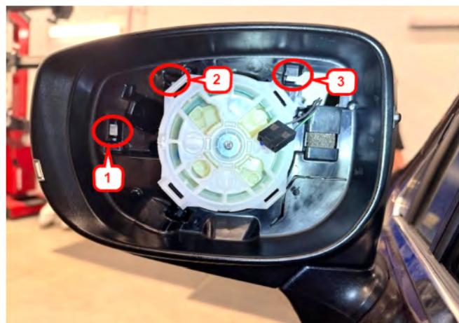
**TIP:** A plastic trim tool can be used to help separate the mirror cover and mirror housing.
