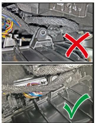
Double check the routing of the harness prior to installing the screws for the cabin air filter cover.
