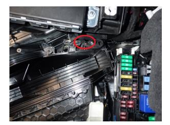
This is where the harness can be damaged when installing the cabin air filter cover screw.
