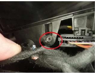
With the harness pulled out of the way, you can see the screw mounting hole for the cabin air filter cover.
