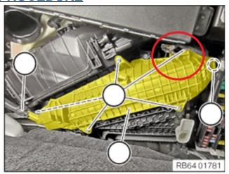
When following Repair Instructions REP **64 31 010** to change the cabin air nanofilter, check the vehicle wiring harness routing (circled) before fastening the plastic cover over the filter.
