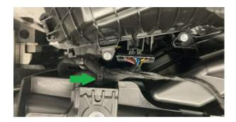
Add a retainer to the harness to prevent it being pinched under the air filter plastic cover.
