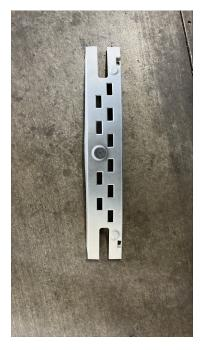
Photo shows the center section of the new front bumper cover that will be removed during installation. This section, if not removed, blocks the FRSF front radar reducing the functionality and causing erroneous behavior.
