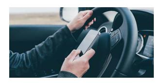
1. Verify the issue is currently present by initiating a phone call during test drive with a paired mobile device. During the call, the call recipient must report that interference in present on the call.
