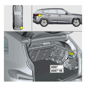
2. Access connector A567\*1B on the VDP and remove pin 1 (1.5 BR). This pin and wire can be tied back to the harness as it will not be used moving forward.
