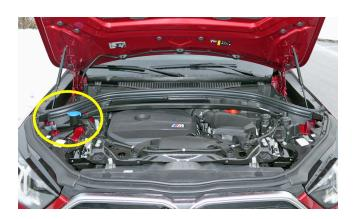
The washer fluid reservoir (filler neck circled) may be leaking, and drains out through the wheel well liner. When the vehicle is parked, a puddle of washer fluid may be present under the right front corner.
