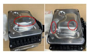
Do not install any part which shows visual damage as shown in the photo or has been dropped from any height.
