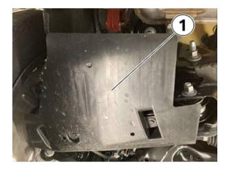
Remove the protective cover (1). NOTE: Tightening torque for screw is 3 Nm.
