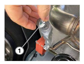
Install the 3 mm washer onto the hanger (1) (use a small amount of sealant to hold the washer to the hanger).
