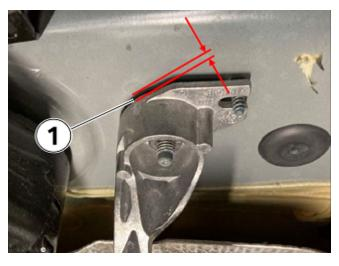
Reinstall the hanger and replace the nut. Tightening torque 19 Nm. There will be a gap between the body and the hanger (1).
