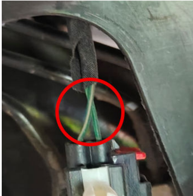
Fig. 5 Area To Inspect For Damaged Wiring
