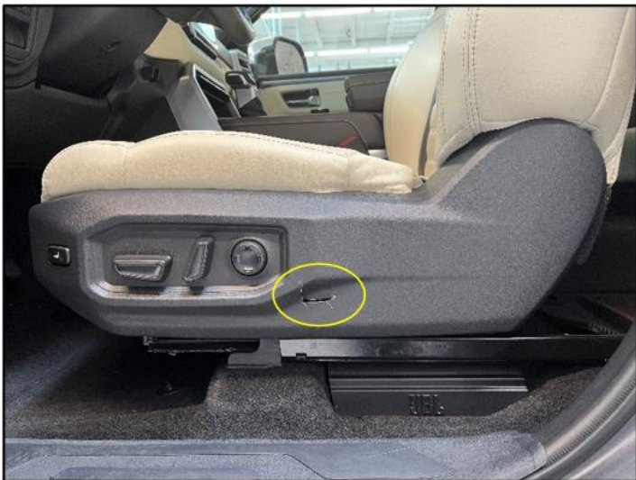
Figure 1: Side shield cracking View
