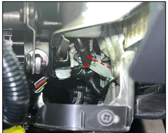
Figure 2: 3 rd clip mis-installed
