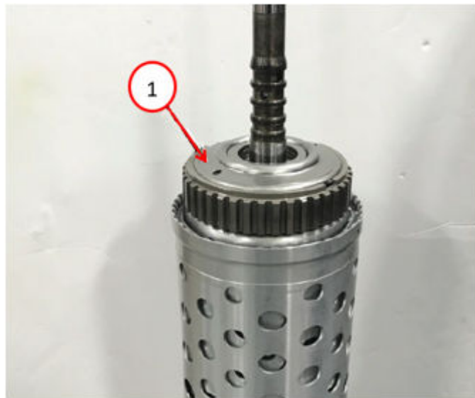
Fig. 32 P1 Annulus/B Clutch Hub Assembly
