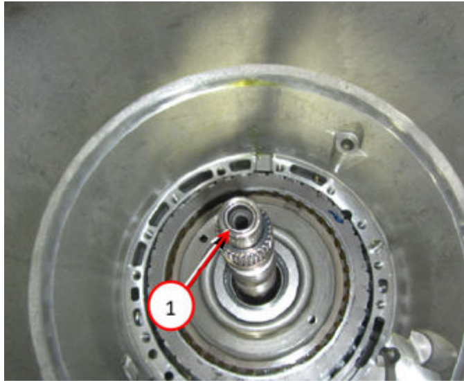
Fig. 35 P4 Annulus Drum Assembly
