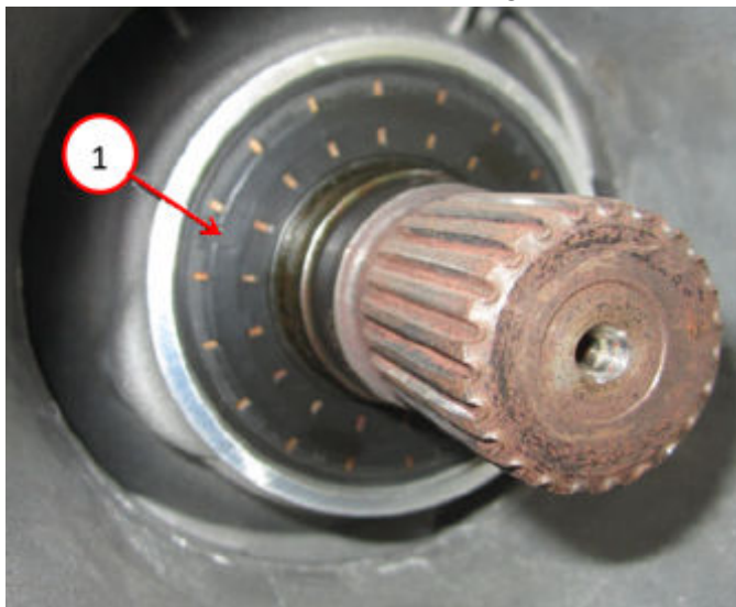
Fig. 51 Transmission Output Shaft Seal Installed
