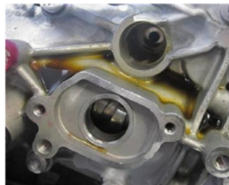
Fault type 2: Cylinder head cover leaking
