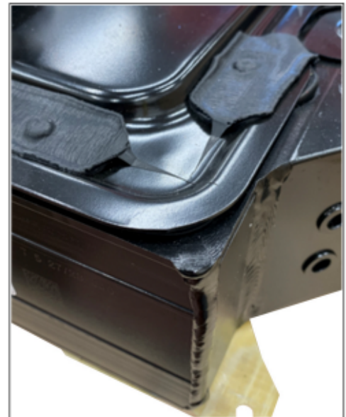
Detailed view of welded seams (sample representation at rear right frame corner)
