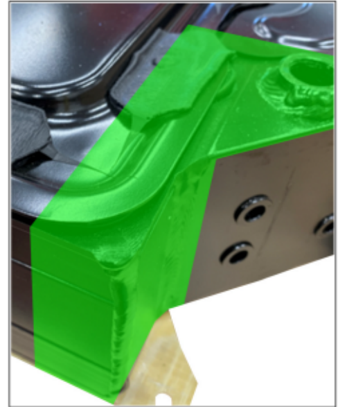
Detailed view of cleaned weld seams (representation of cleaned area in green)
