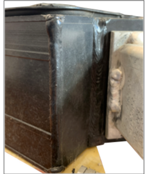
Side view of weld seams (sample representation at rear right frame corner)
