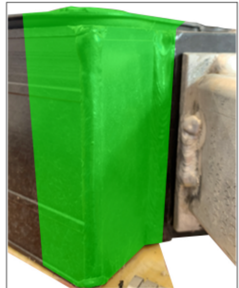
Side view of cleaned weld seams (representation of cleaned surface in green)
