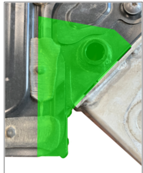
Top view of cleaned weld seams (representation of cleaned surface in green)
